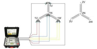
3. Take the secondary cables (clamps) of TRT3x instrument from the primary side of the transformer and connect them to the secondary side of the transformer as shown in the figure below. Perform the test three/four times, using each test voltage. Save all results.
