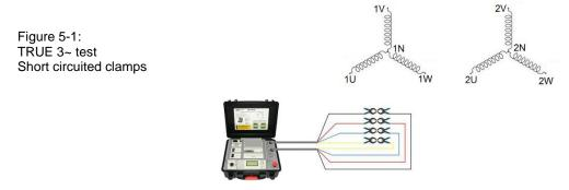
2. Connect the shorted primary and secondary cables (clamps) of TRT3x instrument to the primary side of the transformer as shown in the figure below. Perform the test three/four times, using each test voltage. Save all results.
