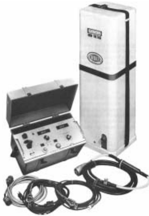
Figure 3: Catalog No. 220163, 160 kV Test
