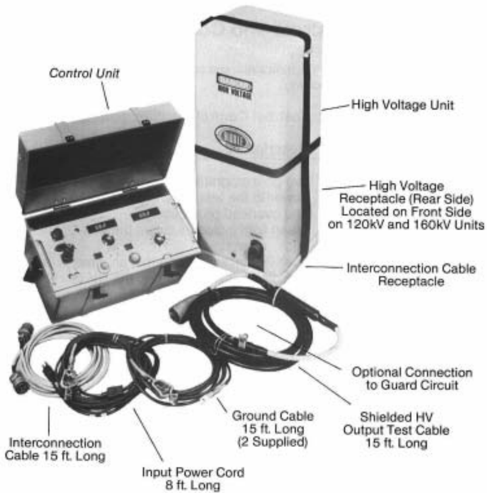
Figure 4: Test Set and Cable Identification
