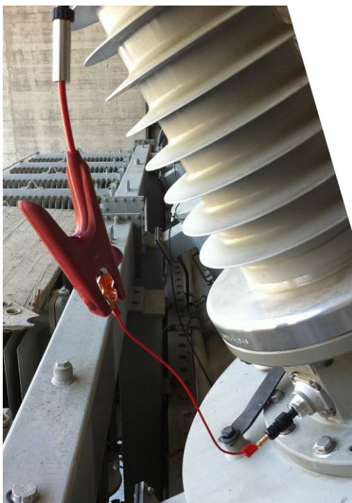
a) Connecting to a bushing test tap using an additional 3 mm cable.
