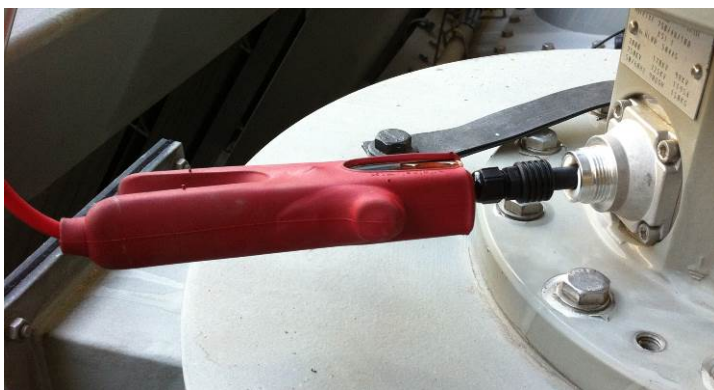
b) Connecting to a bushing test tap using the high voltage clamp.
