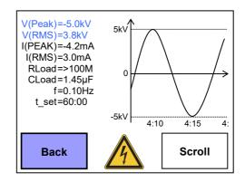
On the right side of the detail view, the test voltage characteristics (AC voltage test) or the characteristics of the leakage current (DC voltage test) are drawn in real time in a diagram. By using the **Scroll** button and turning the rotary encoder, the user can at any time scroll back to earlier time points.
