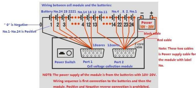
Figure 2.4.4 24cells 2V connection with one cell voltage module.
