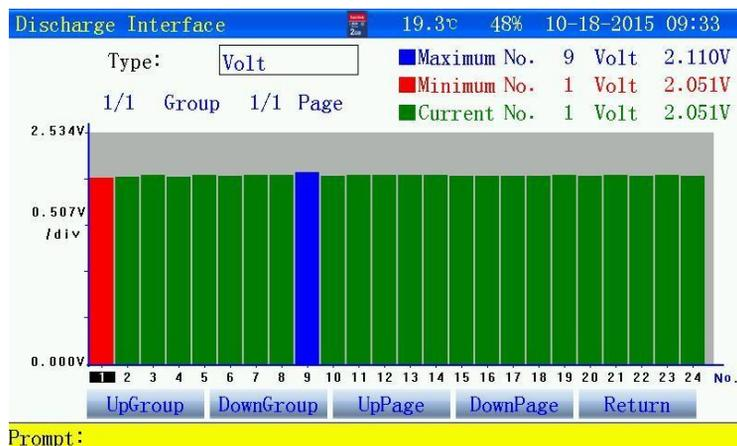
Figure 3.2.4-1 Histogram of cell voltage
