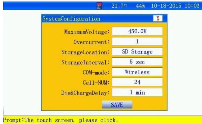
Figure 3.1.2 Interface of time save setup
