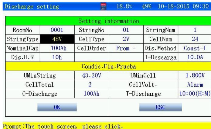
Figure 3.2.2 Interface of setup of discharge parameters
