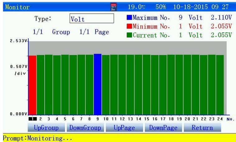
Figure 3.1.4-1 Histogram of cell voltage
