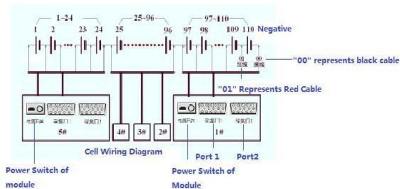
Figure 2.4.4-3 Multi-module connection with the batteries
