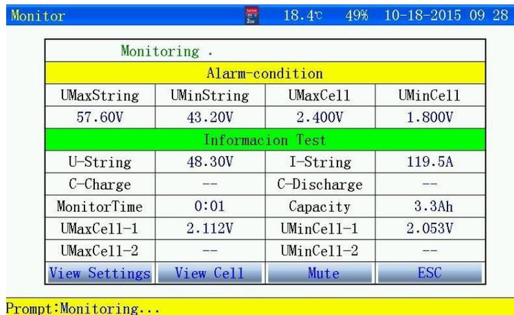
Figure 3.1.3 interface of on line monitoring
