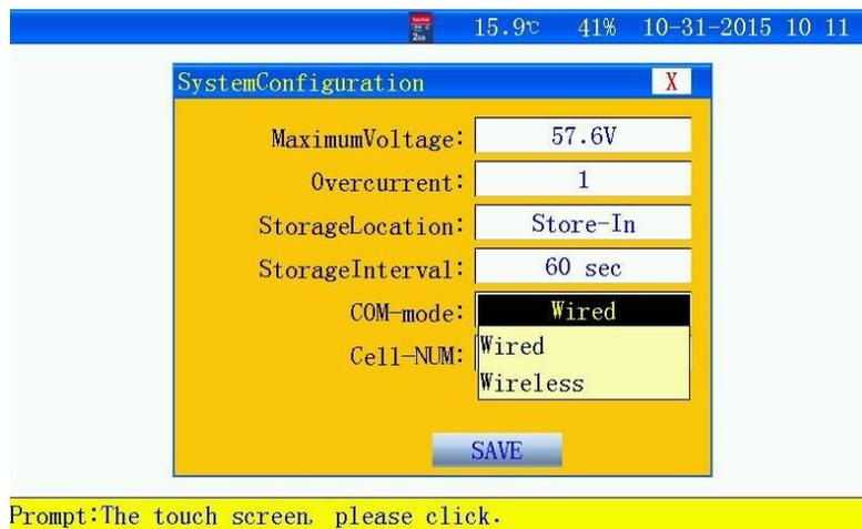
Figure 3.13 Interface of communication setup for the host machine and cell module
