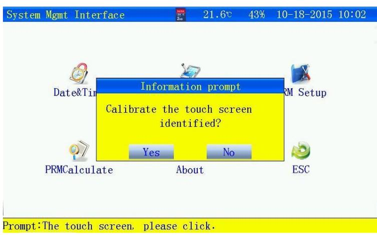
Figure3.7 Calibration of Touch screen
