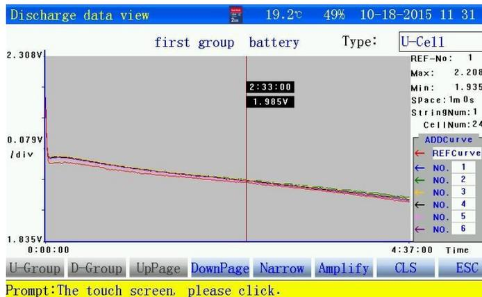
Figure3.5.4-1 Graphic of cell voltage
