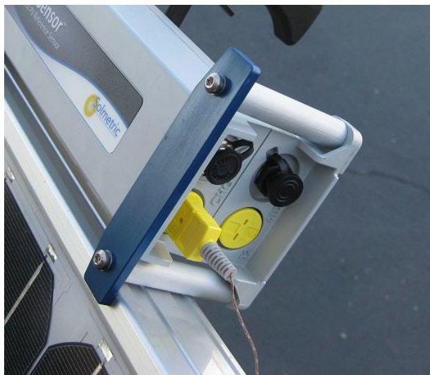
Figure 16. Thermocouple plugged into the TC1 connector.
