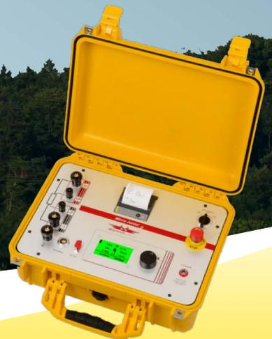
Raytech Digital Micro ohm meter, Micro Junior 2, is designed for a high degree of accuracy to measure very low resistances. It is battery operated with a lithium-ion battery that allows over 2000 test measurements with 10A output without recharging.
