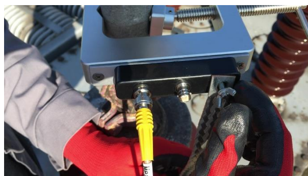
"Measure" lead connection to the large signal clamp
