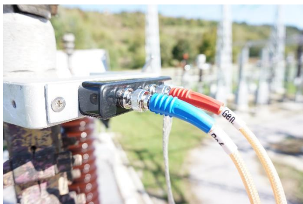
"Generator" and "Reference" leads connection to the large signal clamp
