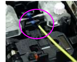
Clamp automatically releases
