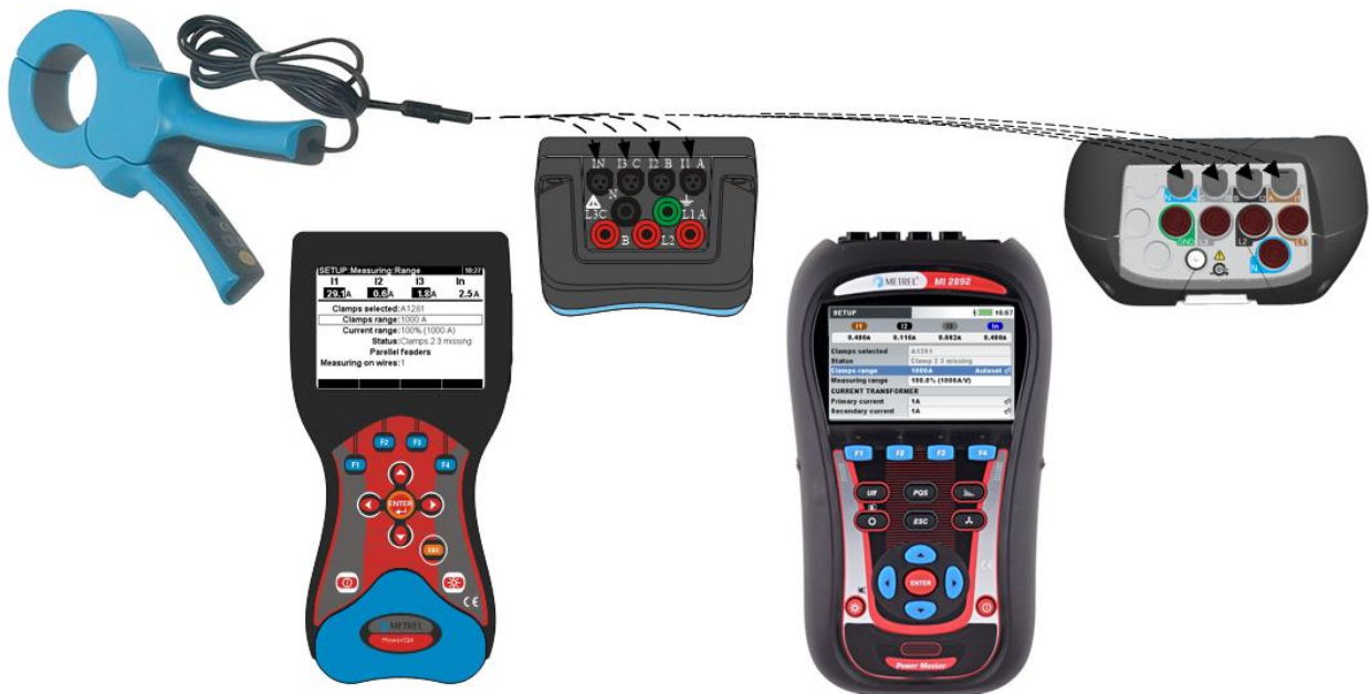
Figure 2: Current clamps A 1281 - connection to the measuring instrument
